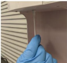
4. Clean the nozzle, pushing the swab as far up as it will go
